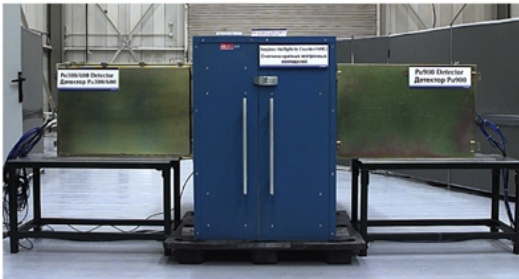
Figure 2. The three AMS/IB detectors. On the left is the Pu300/600, a HRGS system. In the center is a NMC. On the right is the Pu900.
