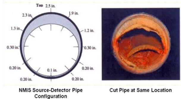
**Figure 1. Image of material in processing pipe.**
