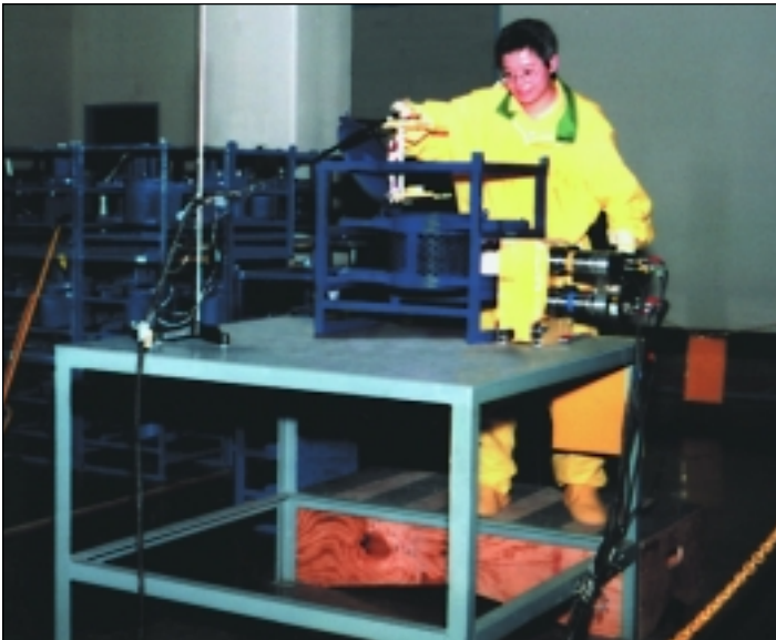
The equipment setup for verifying HEU metal at the Y-12 Plant in Oak Ridge, Tennessee. The ^{252}\text{Cf} source is located near the part. The uranium mass and enrichment of the HEU metal in birdcages were determined to within \pm 2\% .
