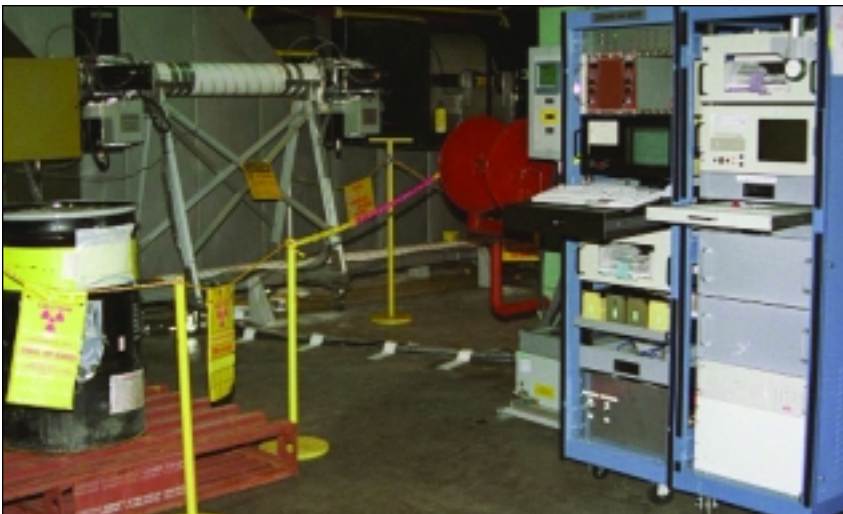
The Blend-Down Monitoring System (BDMS) consists of a flow monitor and an enrichment monitor for each pipeline in the Russian down-blending facilities.
