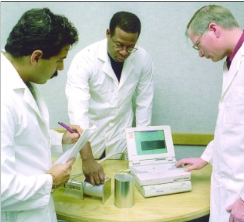
The portable NDA equipment used for measuring the ^{235}\text{U} enrichment of uranium in containers.
