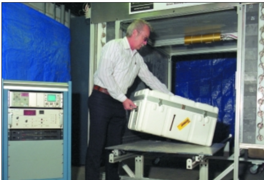
The Active Interrogation Package Monitor can detect the presence of special nuclear materials in a few seconds even when the material is heavily shielded.
