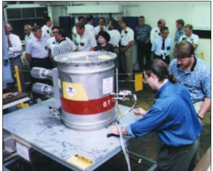
Russian visitors watch a demonstration of the active interrogation technique. The ^{252}\text{Cf} source and detectors are located around a container with a weapon component inside.
