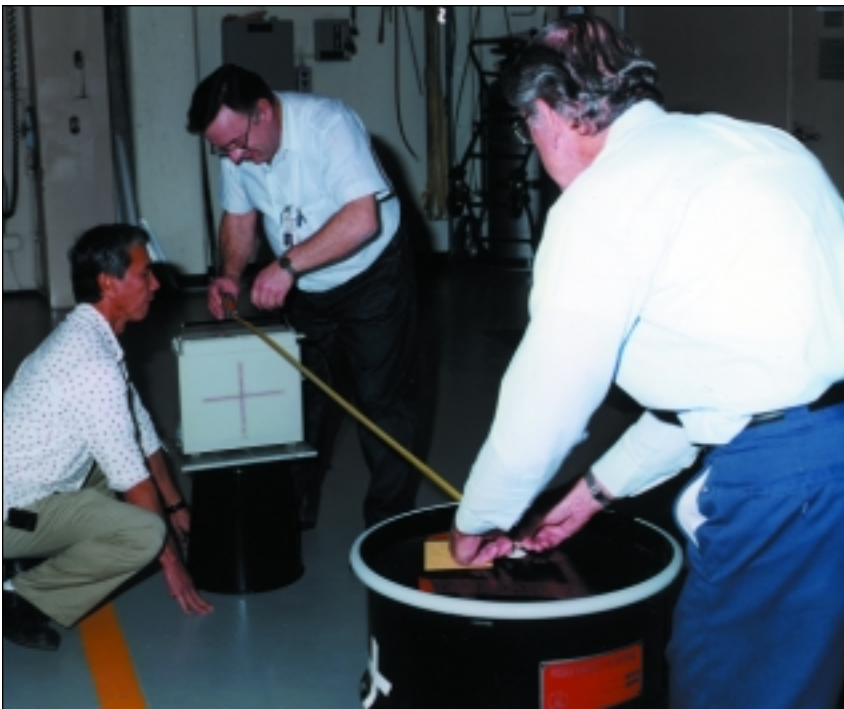
Vayacheslav Yanov of the Russian Research Institute of Pulsed Techniques (center) prepares to make a plutonium mass estimate using a SRPS7 neutron detector during the 1994 joint experiments with Los Alamos and Lawrence Livermore National Laboratories.
