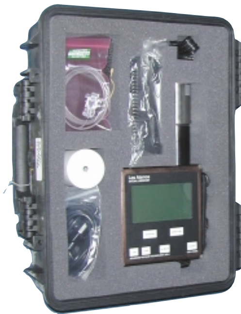
A RANGER-PLUS system (lower right) and its accessories in its rugged transport case. This system is a low-resolution spectrometer that can detect and identify plutonium.
