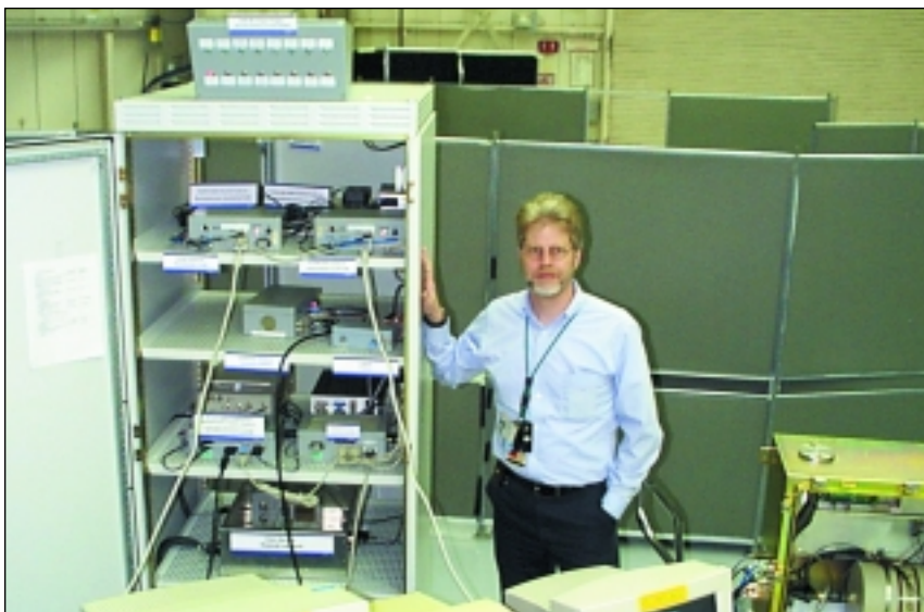
A rack shields the electronic components as part of an information barrier incorporated into the Fissile Material Transparency Technology Demonstration, held at Los Alamos National Laboratory in August 2000.
