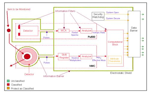
The system consisted of one high-purity germanium (HPGe) detector and one small Neutron Multiplicity Counter (capable of holding a 1-gallon drum). The HPGe detector had a mechanical iris to keep the gamma ray count rate constant independent of the source being measured. The entire system was enclosed in a series of shielded enclosures connected with shielded cables. Attributes were determined sequentially, first using the gamma system, then the neutron system.<sup>8</sup>
