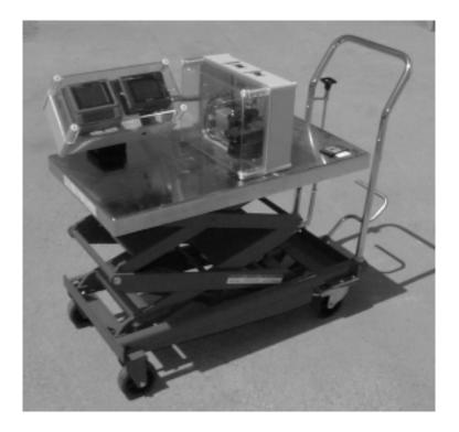
Figure 3: The Cart-Cam used by the IFMS for close-up video images of ITID installation and removal from individual containers.
