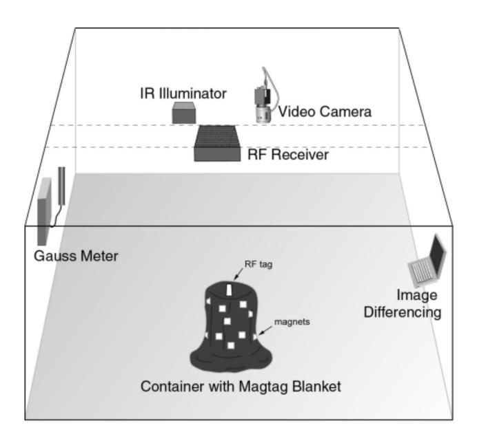
Figure 5: A schematic of the Magazine Transparency System (MTS) showing the primary components.
