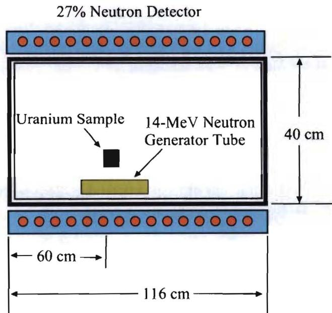
Figure 6. Typical setup for delayed neutron reinterrogation measurements.
