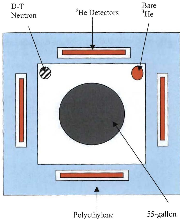
Figure 4. A top view of a typical DDA setup.
