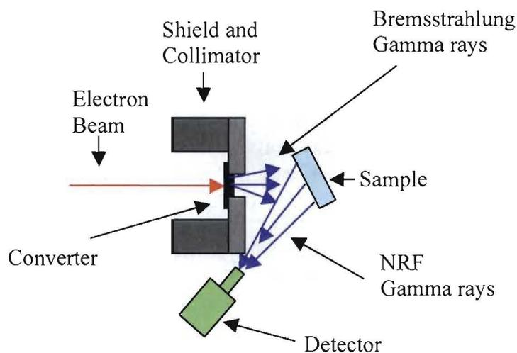
Figure 1. A typical NRF experimental arrangement.
