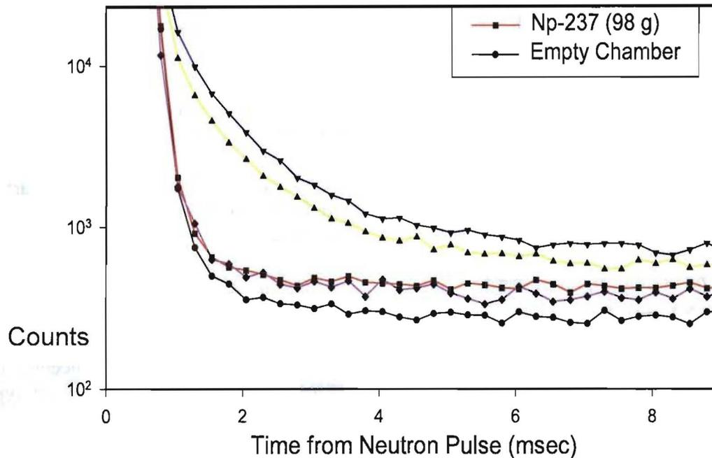
Figure 5. Time history of shielded detector response with (upper curves) and without (lower curve) SNM.
