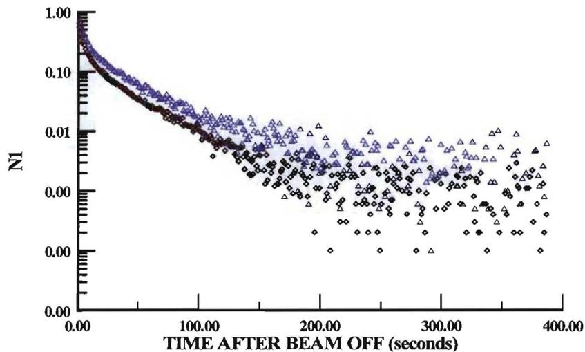
Figure 7. Delayed-neutron-driven response for 91% enriched uranium (upper curve) and 0.2% depleted uranium (lower curve).
