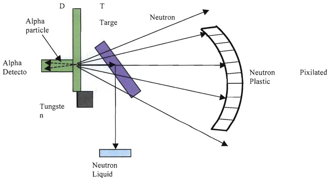
Figure 8. A typical associated particle experimental setup.
