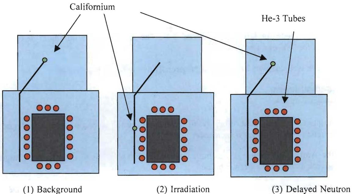
Figure 3. Operation of a californium shuffler.
