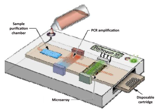
Figure 7. Sketch of a possible instrument for biological weapons verification.
