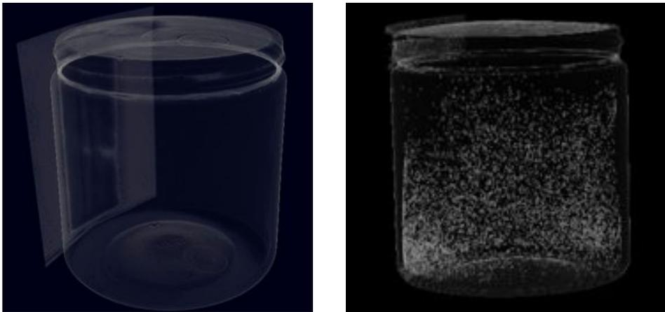
Figure 4: CT scan of detector exposed to 1 Gy of 6 MeV  $\gamma$  rays (left). CT scan of same detector exposed to 2.5 mSv of AmBe neutrons (right).
