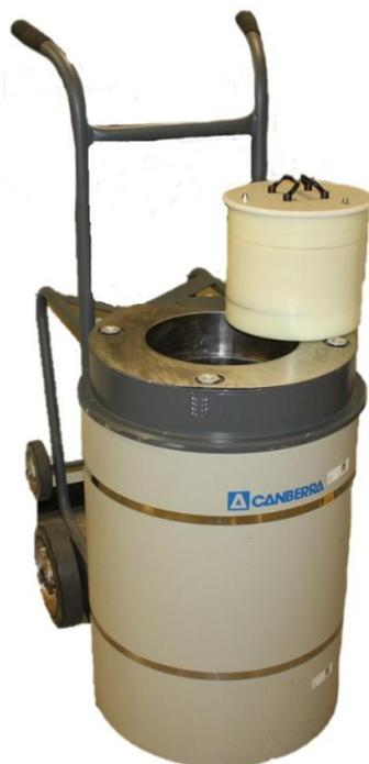
*Figure 1. A photograph of the ORNL LV-AWCC. The top-plug is shown removed and is resting on the electronics enclosure.*
