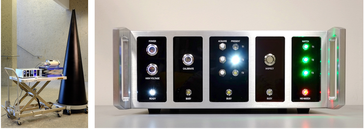
Figure 4: Typical experimental setup with mockup warhead (left) and Information Barrier Experimental (IBX) during initialization sequence (right).
