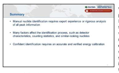
We have discussed the general process of nuclide identification. Pattern recognition is dependent on the experience of the spectroscopists, while peak-based identification requires an accurate energy calibration and a thorough explanation of all features in a spectrum. We discussed ten causes of isotope misidentification, although there are more, particularly with
