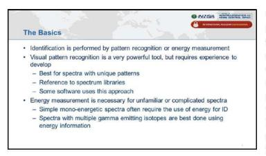
Visual pattern recognition is analogous to recognizing your friend's face. If the unknown spectrum looks like one you have seen before, you may be able to quickly identify it. However, it is also easy to be fooled because many radionuclides have similar spectra. Measuring peak energies and comparing them with reference data is necessary when you do not
