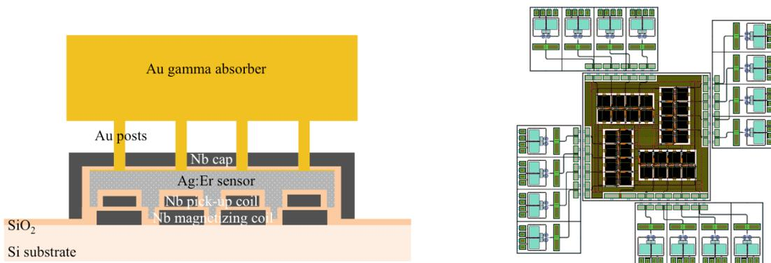
Fig. 4 (left): Schematic cross section of the MMC with the Au gamma-ray absorber supported on top of the Ag:Er sensor by Au posts. Current in the lower Nb coil magnetizes the Er spins in the Ag:Er sensor, and sensor heating by gamma-rays induces a signal in the upper Nb pick-up coil that is coupled into the SQUID preamplifier. Fig. 5 (right): Layout of a central 4x8-pixel MMC array, surrounded by four chips with 4 SQUID preamplifiers each.
