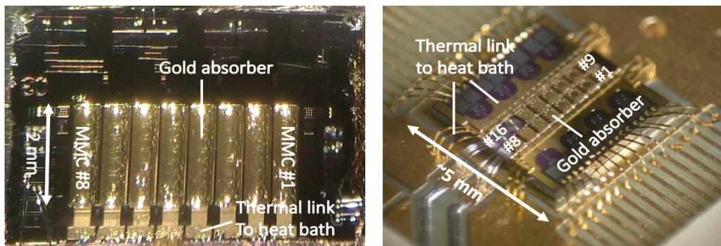
Figure 6: MMC gamma detectors developed at the Kirchhoff Institute of Physics (KIP) at Heidelberg University (left) and at the University of New Mexico (UNM) (right).
