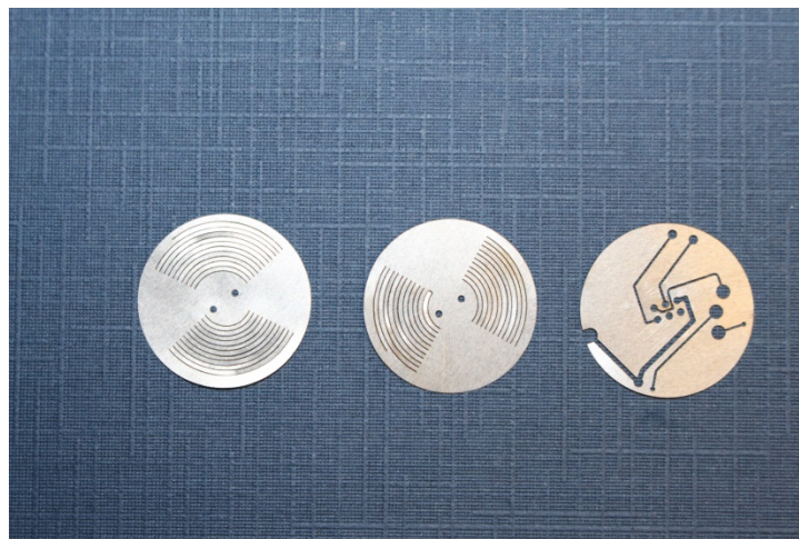
Figure 5: Masks. (Left and center) tamper planes use two separate spiral patterned masks. (Right) mask for circuit board electrical connections.
