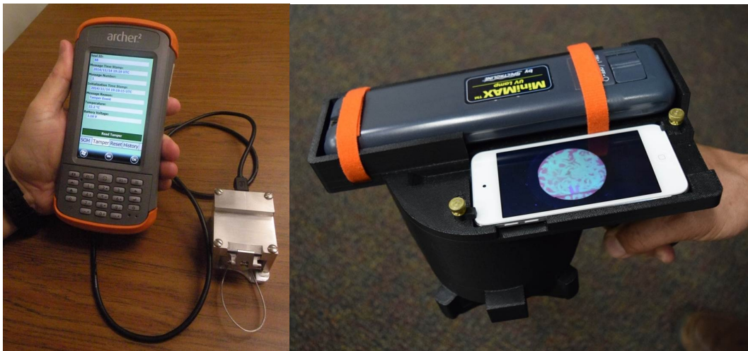
Figure 9: (Left) SRNL handheld standalone reader with seal inserted in module, (Right) Ceramic Seal Coatings Reader.
