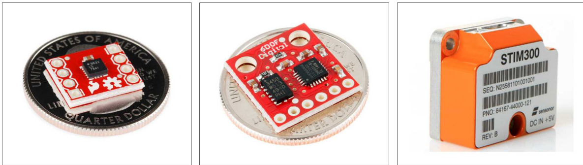
Figure 4. Candidate components for use in the motion-detection subsystem Triple-axis accelerometer (left) and two inertial measurement units (center and right). Image credit: Sparkfun and Sensoror.
