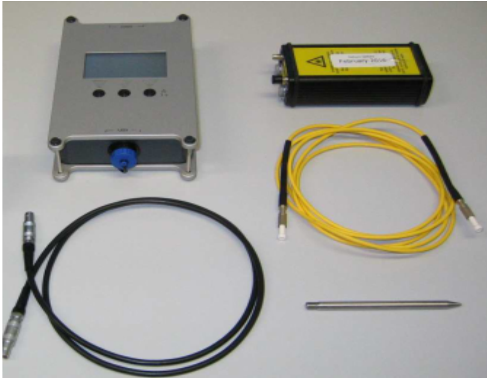
Figure 5. Equipment used by an operator when applying EOSS seal: ESI (top left); EOSS seal (top right); Interface-to seal/camera cable (lower left); fiber-optic cable for EOSS (middle right); Fiber-optic guiding needle (bottom right). Source: (Jussofie, van Bevern, et al. 2014).
