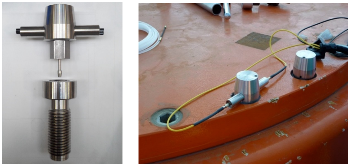
Figure 2. Ultrasonic Optical Sealing Bolt (left); installed on CASTOR storage cask with EOSS (right)
