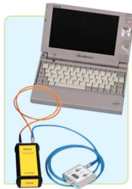
Figure 14: EOSS seal (bottom yellow item) with reader (laptop). (Courtesy Canberra, www.canberra.com )
