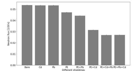
Figure 3: Different shielding and corresponding neutron fluxes.
