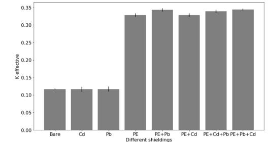
Figure 2: Different shielding and corresponding  $k_{\text{eff}}$ .
