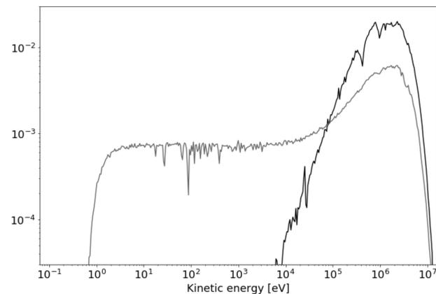
Figure 1: Comparison of bare (black) and 5 cm Polyethylene, 0.11 cm Cadmium, 1 cm Lead shielded (gray) SF neutron spectrum.
