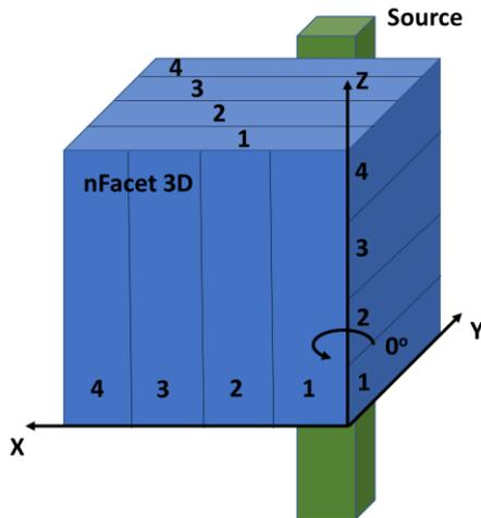
Figure 4. Schematic drawing of the detector. This is the so-called 0 degree measurement orientation.
