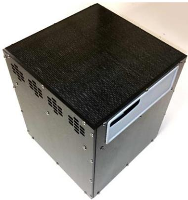
Figure 1. nFacet 3D detector. Weight: 16 kg. Size: 25 x 25 x 27 cm<sup>3</sup>
