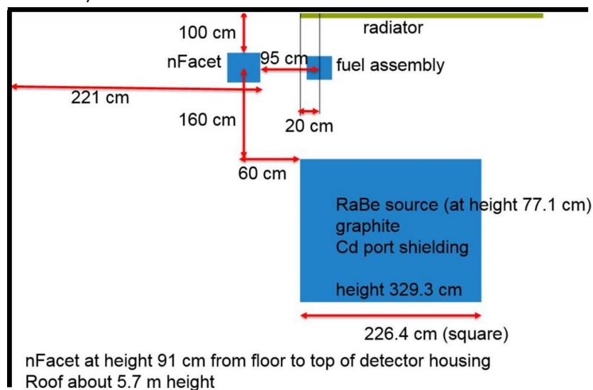
Figure 3. Schematic drawing of the measurement room
