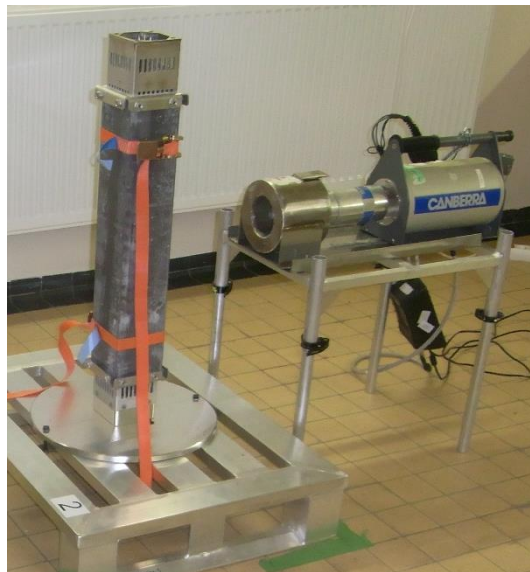
Wide collimator aperture for general measurements
