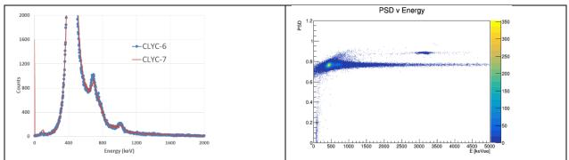
Above are presented gamma ray spectrums for configuration 11 (sample with 96% of <sup>239</sup>Pu). Due to midresolution capability of the gamma detectors, results are combination of peaks originating from U and Pu isotopes as well as from <sup>241</sup>Am. System's resolution was not good enough, and therefore was not able to identify peaks due to Pu or U.
