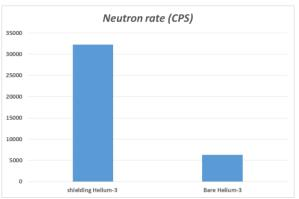
By comparing the neutron count rate for configurations with the He-3 detectors shielded and unshielded, one can qualitatively asses the neutron energy spectrum. For sample with 62% of <sup>239</sup>Pu, the count rate drops significantly when a bare He-3 detector is used, indicating the presence of fast neutrons.
