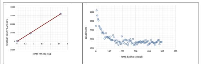
(Left) Shielded He-3 (fast neutrons) counting. (Right) Example of neutron coincidence and Rossi-Alpha distribution for configuration 3 with 62% of <sup>239</sup>Pu. Neutron count rates are linearly proportional to <sup>239</sup>Pu mass of the sample (left) and are confirmed to originate from a fission source by observing the typical Rossi-Alpha distribution (right).
