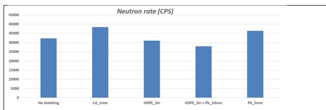
Neutron count rate for different shielding configurations are shown above. Count rate is observed to increase when Pb or Cd shielding materials are used. We suspect this is due to gamma rays generated by interaction of fast neutrons with these shielding materials, which leads to pile-up providing signals above threshold.
