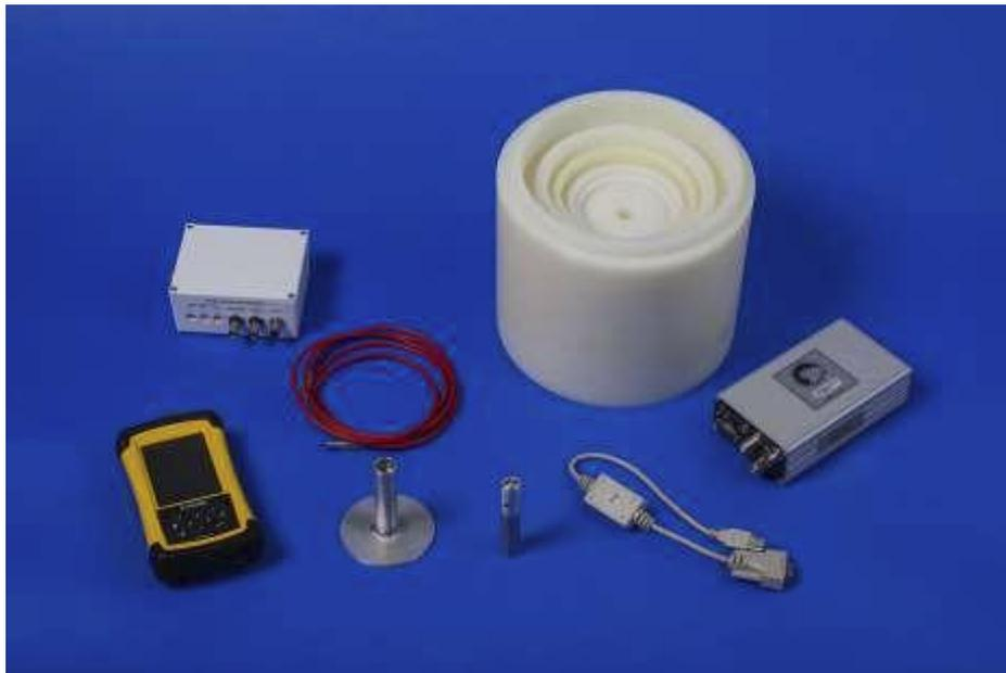
Figure 1. Principal components of the nested neutron spectrometer
