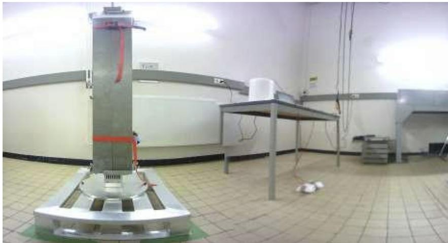
Figure 2. 61-pin assembly with HDPE/Cd shield (on the left); Nested neutron spectrometer with all moderators (on the table) at SCK•CEN (Be)
