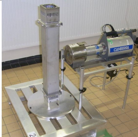
Narrow collimator aperture and close geometry for measuring isotopic ratio distribution
