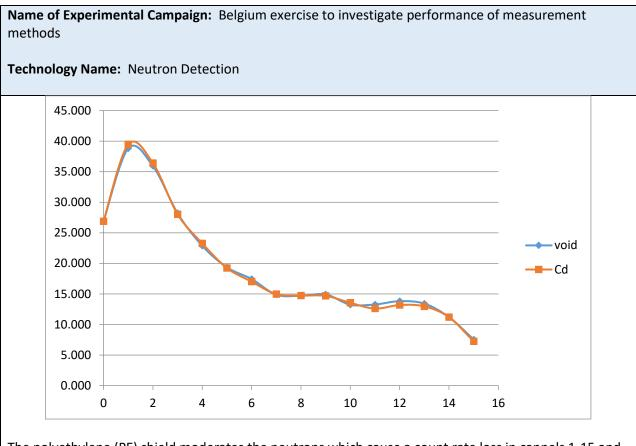
The polyethylene (PE) shield moderates the neutrons which cause a count rate loss in cannels 1-15 and a gain in channel 0. Subsequent Cd shield cause a sharp drop in channel 0 and has no influence for channels 2-15.
