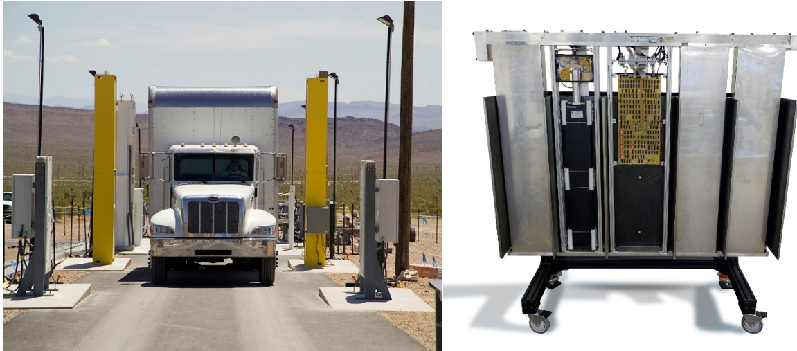
Figure 1: Vehicle portal monitor (credit: NNSA Nevada Site Office Photo Library); hallway Portal Monitor for Authentication and Certification (PMAC) showing two modules with tamper-indicating enclosure removed (credit: Sandia National Laboratories)
